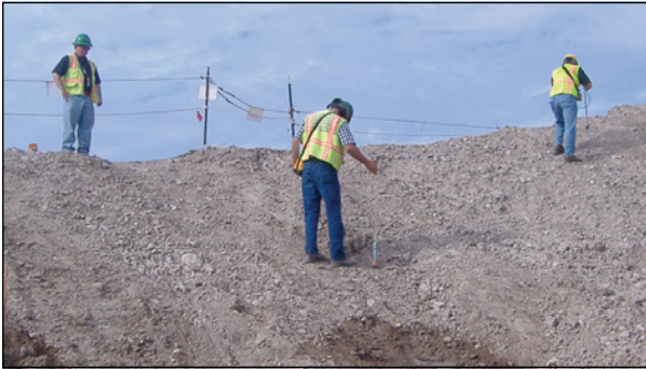
Site Survey of Below-Grade Areas Assures site is free of contamination (NRC file photo)
