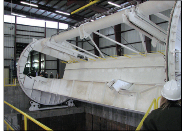
Railcar Roller at Clive This equipment allows for fast, efficient unloading of material
